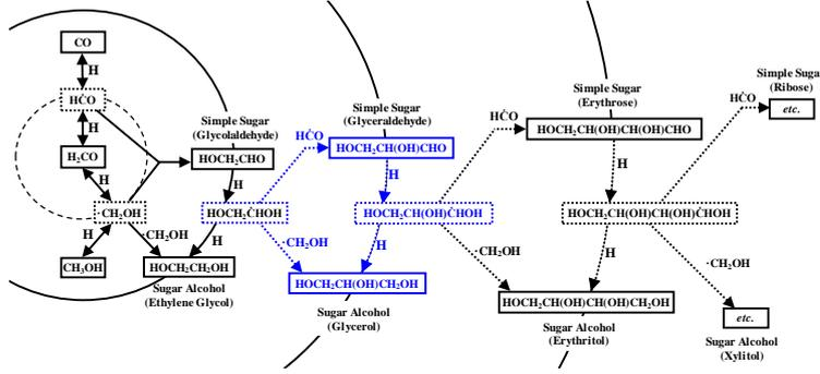
**Figure 5.** Reaction scheme leading to complex sugars in ices at low temperatures (10-15 K), without the need for UV radiation or cosmic rays. Figure from Fedoseev et al. (2017).
